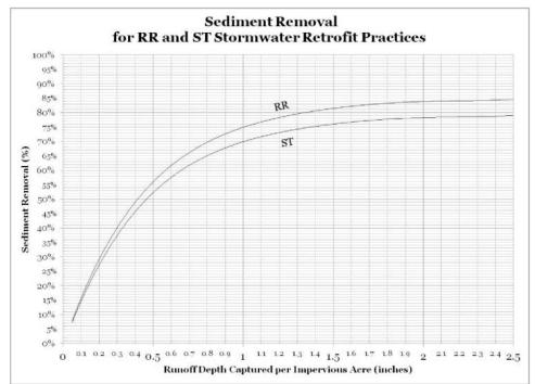
Figure 3 - Retrofit Pollutant Removal Adjustor Curve for Total Sediment (Suspended Solids)
