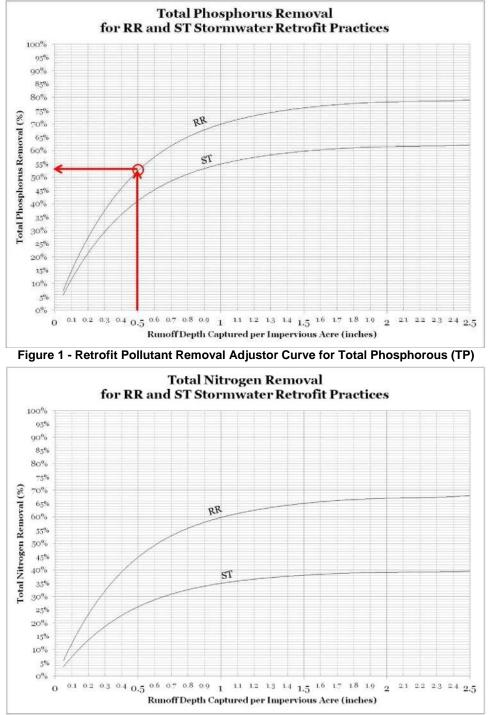
Figure 2 - Retrofit Pollutant Removal Adjustor Curve for Total Nitrogen (TN)
